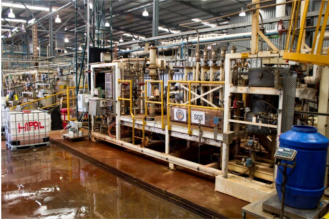
Figure 6: Scandium Solvent Extraction pilot plant (June 2012)
