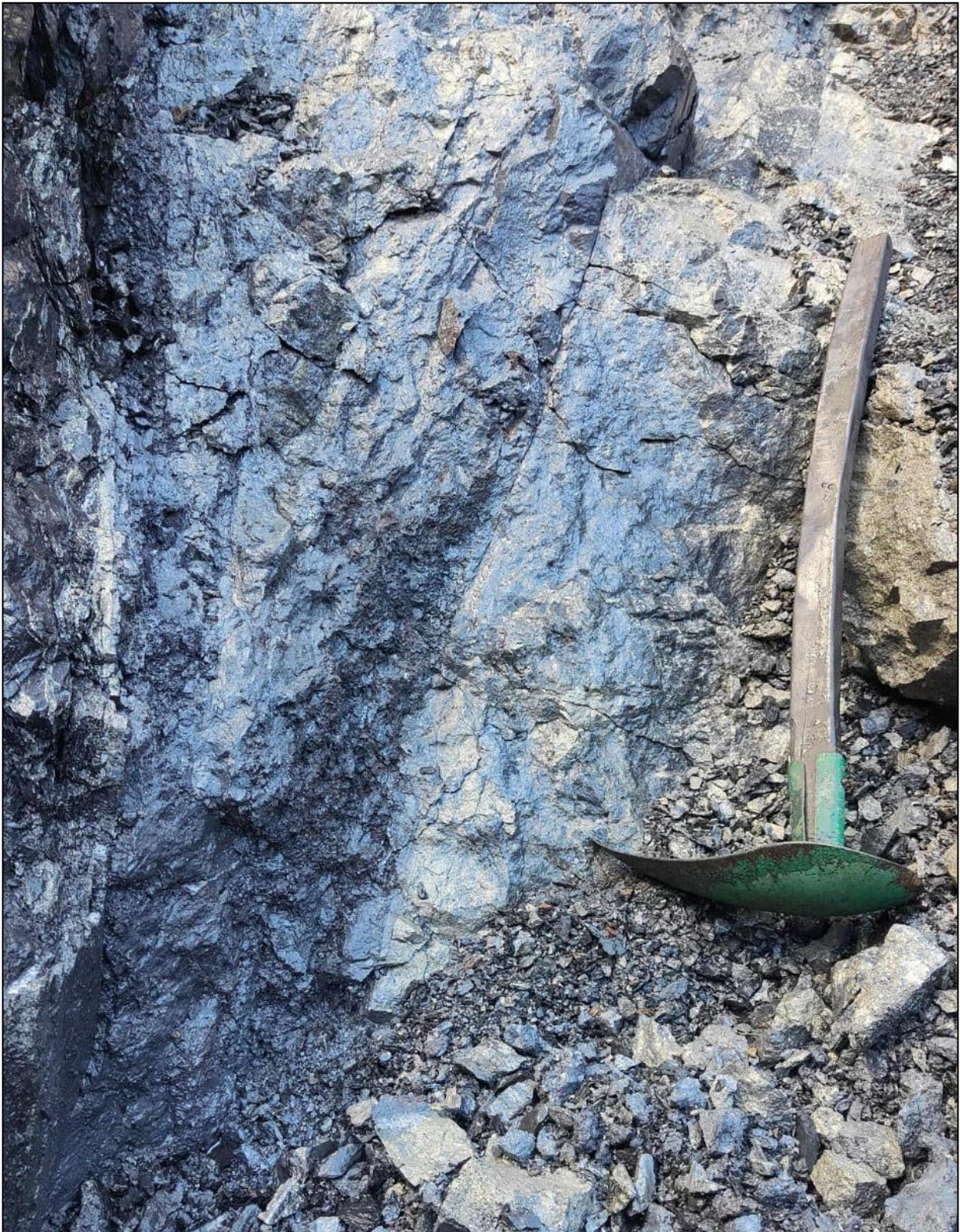
Figure 10. Montezuma antimony-silver-lead deposit – Trench grab sample SGD+25, assays returned 24.5% Sb, 501g/t Ag and 39.8% Pb
